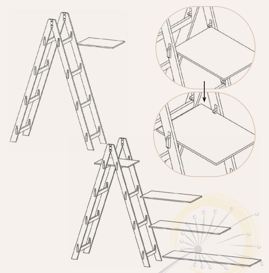
7. Slide shelves into the unit, resting on the supports. The shelves will be fitted through the slots of the supports.
